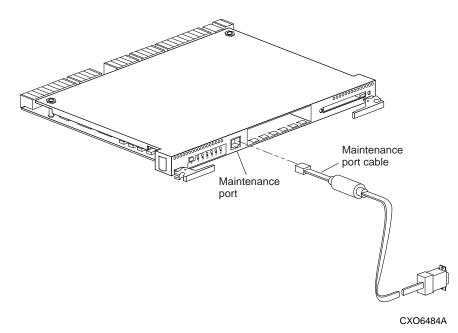
Figure 2–5. PC/Terminal to Maintenance Port Connection
